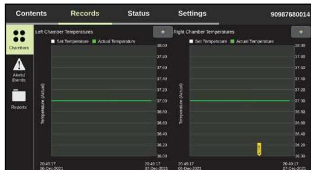
2. Tap the plus (+) icon on the top right of each incubation chamber graph to show only the selected chamber. Tapping the magnify +/- will zoom/expand the time scale.
