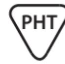
This symbol on the label indicates that this device contains phthalates. Specific phthalates contained in the device are identified beside or below the symbol by the following acronyms:
